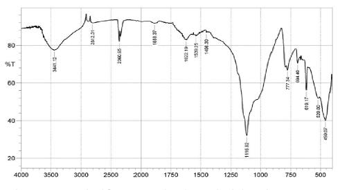
Fig. 2. FTIR analysis of SNPs synthesized from Bridelia ferruginea bark extract
