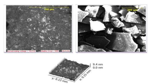
Fig. 3. SEM micrographs of SNPs synthesized from Bridelia ferruginea bark extract
