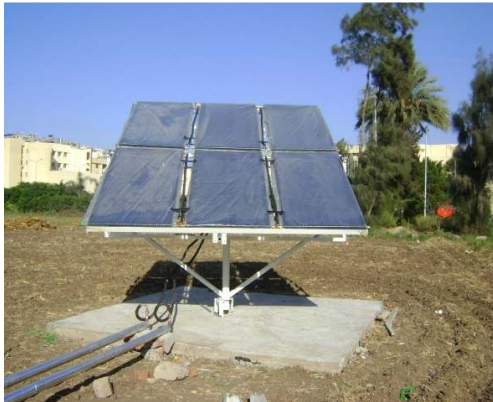
Fig. 1. Solar collectors array, with a total surface area of 12.0 m 2 and mounted on a movable frame
