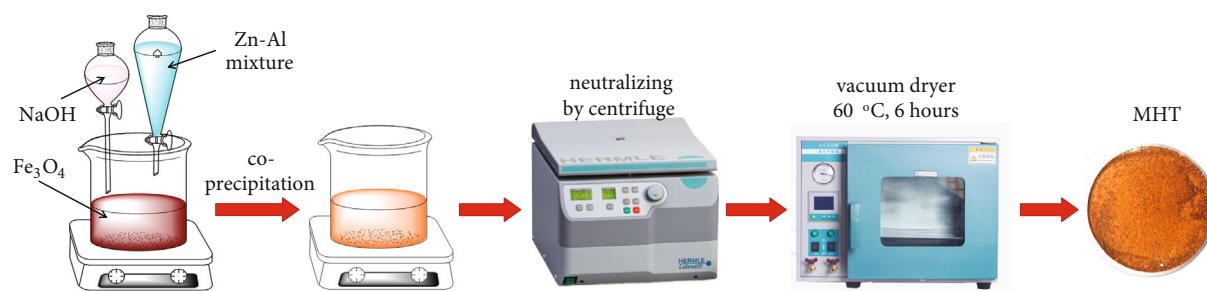
FIGURE 1: Schematic illustration of synthesis steps for MHT.
