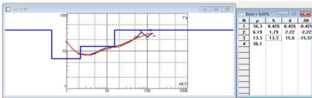
Fig. 16. VES station 11 shows graph of apparent resistivity against electrode spacing
