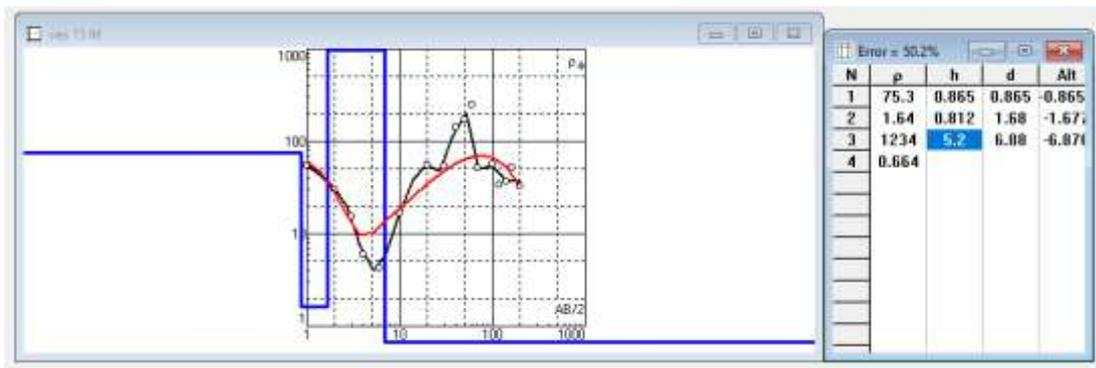
Fig. 20. VES station 15 showing the graph of apparent resistivity against electrode spacing
