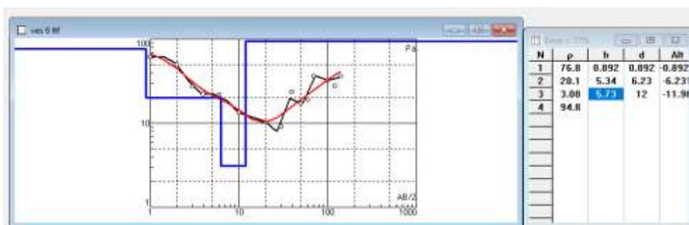
Fig. 11. VES station 6 showing the graph of apparent resistivity against electrode spacing
