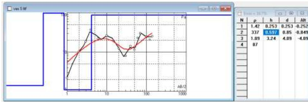
Fig. 10. VES station 5 showing the graph of apparent resistivity against electrode spacing
