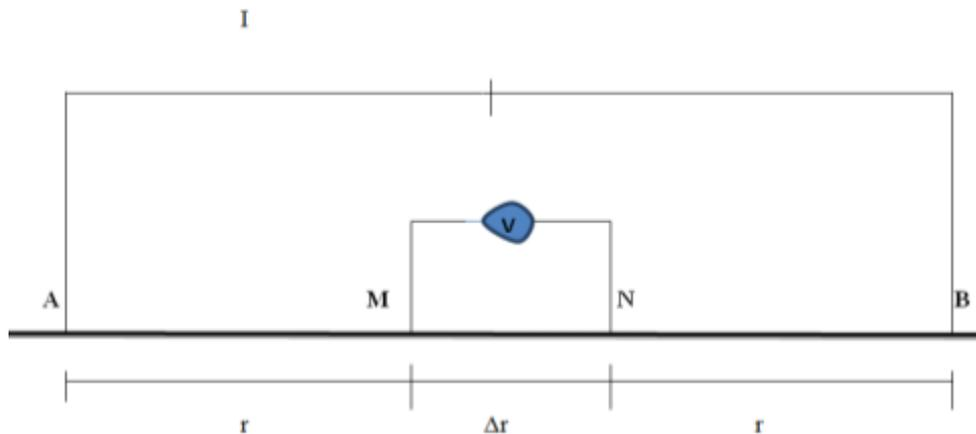
**Fig. 4. Configuration of Schlumberger Array**
