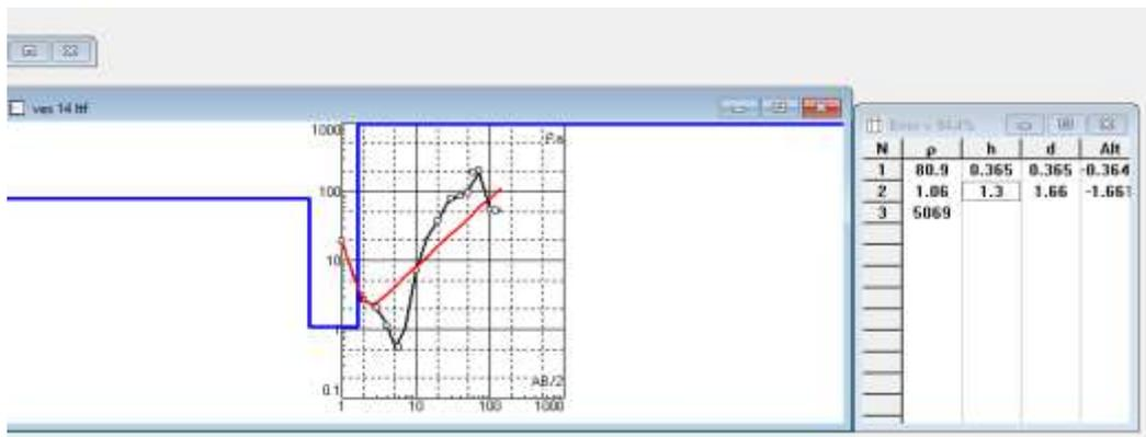
**Fig. 19. VES station 14 showing the graph of apparent resistivity against electrode spacing**
