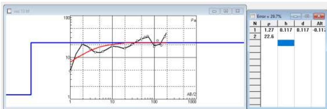
**Fig. 18. VES station 13 showing graph of apparent resistivity against electrode spacing**
