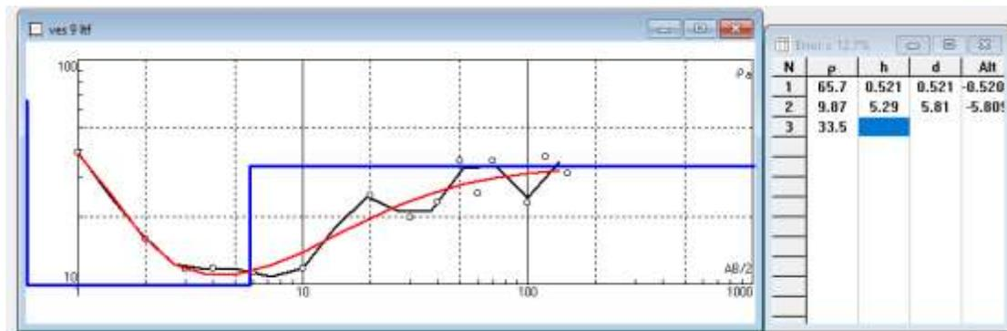
Fig. 14. VES station 9 showing the graph of apparent resistivity against electrode spacing
