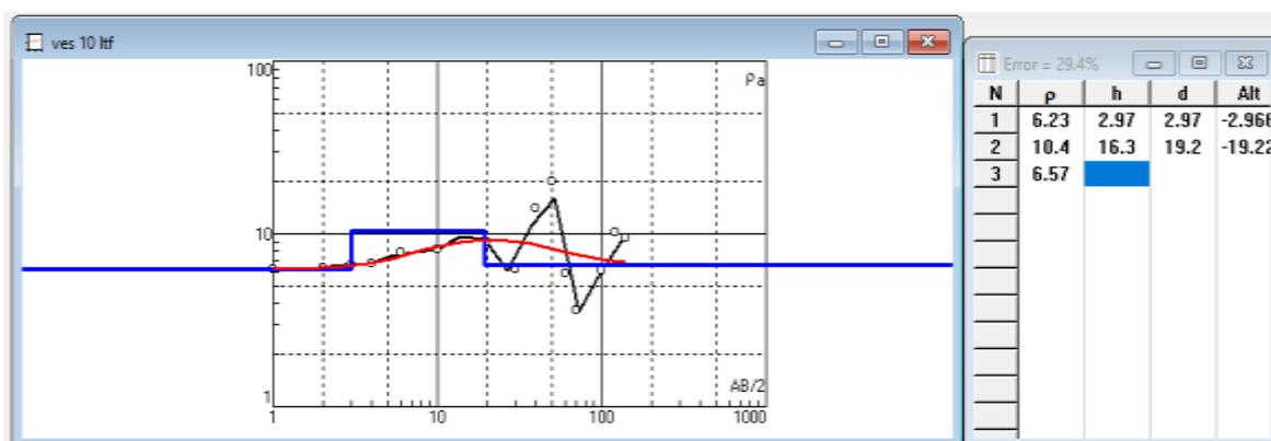
Fig. 15. VES station 10 showing the graph of apparent resistivity against electrode spacing
