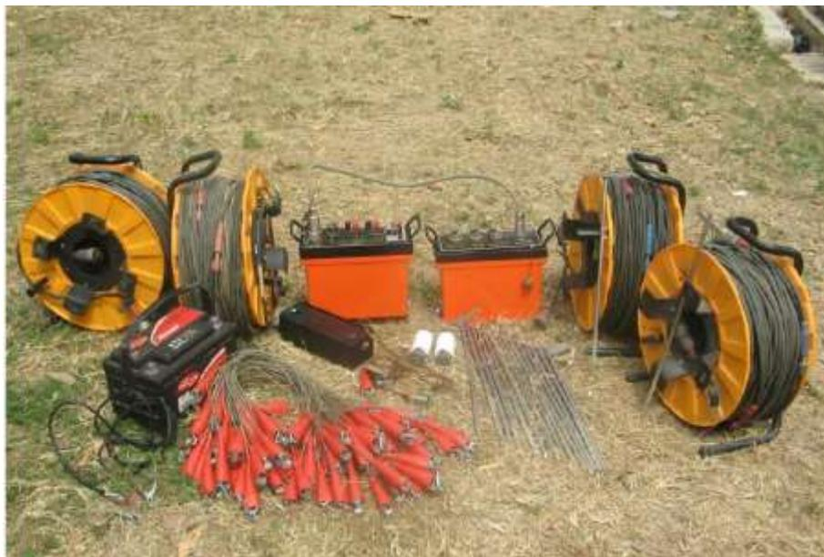
Plate 1. Electrical resistivity equipment and other accessories
