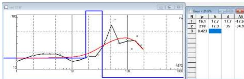
Fig. 17. VES station 12 showing the graph of apparent resistivity against electrode spacing
