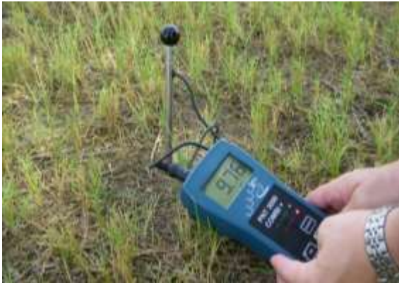
Fig. 3. Direct measurement of soil salinity using salinity probe
