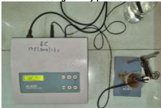
Fig. 4. Indirect measurement of soil salinity using EC meter
