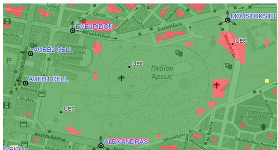
Figure 5. Unloaded and loaded URLLC traffic areas due to OF propagation.
