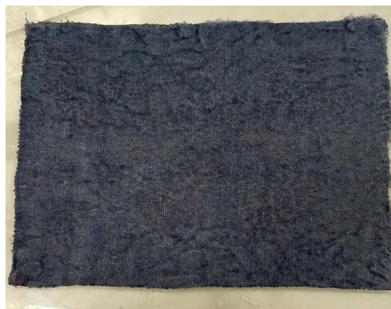
Figure 3. Surface treatment of bamboo fabric with NaOH.
