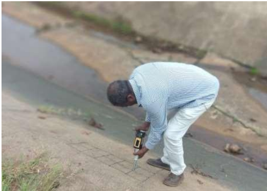
Fig. 9. Conducting rebound hammer test
