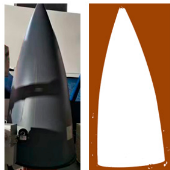
Figure 3. An aircraft radome and its 3D scanned point cloud of aircraft radome.
