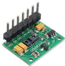
Fig. 4. Max30100 pulse oximeter and heart-rate sensor [14]
