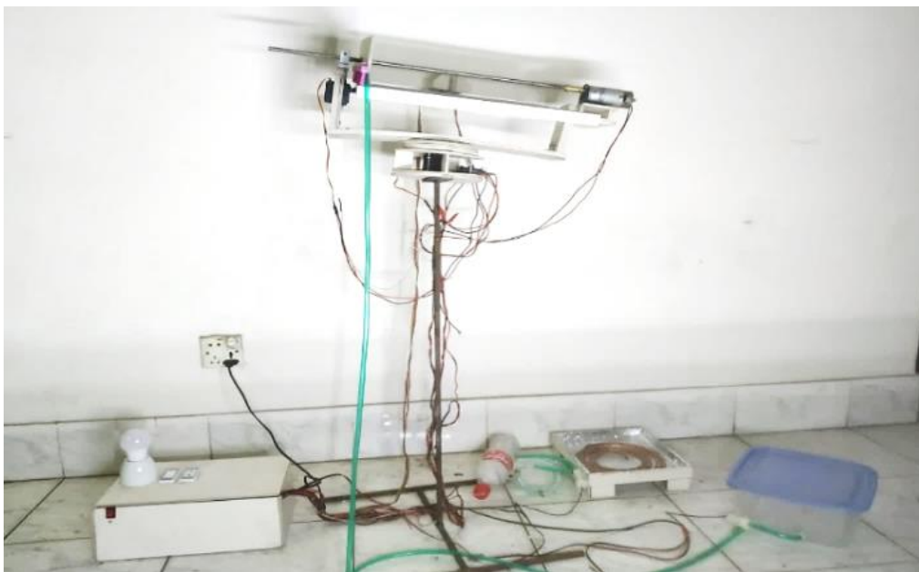
Fig. 10. Implemented dual-axis solar tracking, panel cleaning, and power management system project
