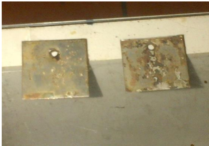
Fig. 2. Shows the effect of UV on NaCl after cleaning
