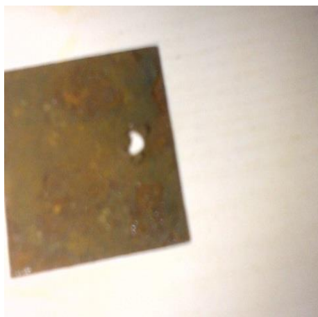
Fig. 6. Shows the effect of UV on NaCl after one week after cleaning
