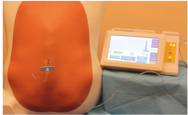
FIGURE 1: Study settings: the CompuFlo® epidural instrument and the epidural simulator.
