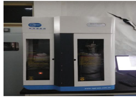
FIGURE 2: Hsorb-2600 high-temperature and high-pressure gas adsorbent instrument.
