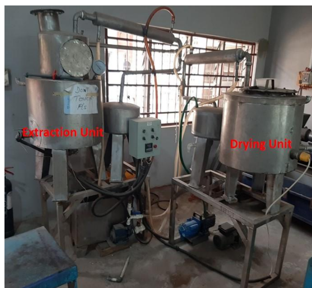
Fig. 4. The macroscopic image of the fabricated natural dye extractor and dryer machines
