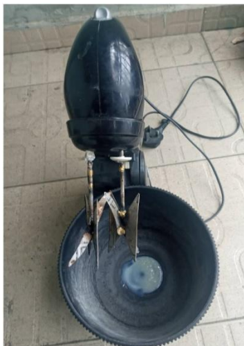
Plate 2. Mixing the slurry with the TETE blade stirrer arm
