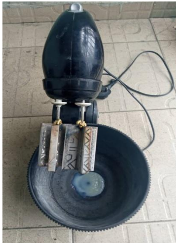
Plate 1. Mixing the slurry with the two z-blade stirrer arm
