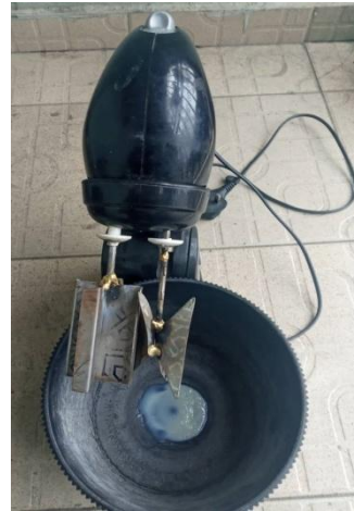
Plate 3. Mixing the slurry with the two Z - TETE blades hybrid stirrer arm
