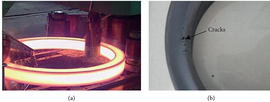
FIGURE 17: Cracking of ring in the hot ring rolling experiment. (a) Hot ring rolling experiment. (b) Cracking of the ring.
