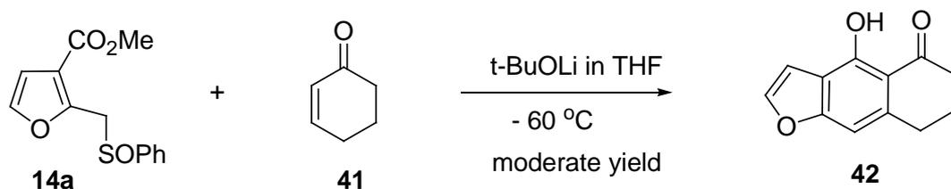
**Scheme 10.** Synthesis of dihydro naphtho[2,3-*b*]furanone moiety **42**.
