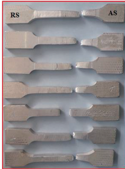
FIGURE 9: Fractography of tensile test specimen.
