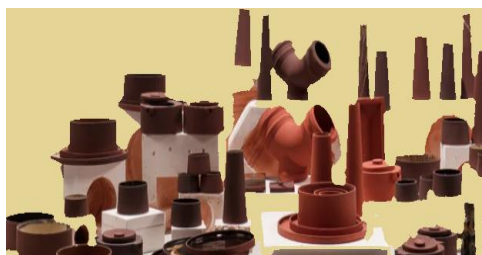
Fig. 2. The ceramics produced from red mud and clay minerals
