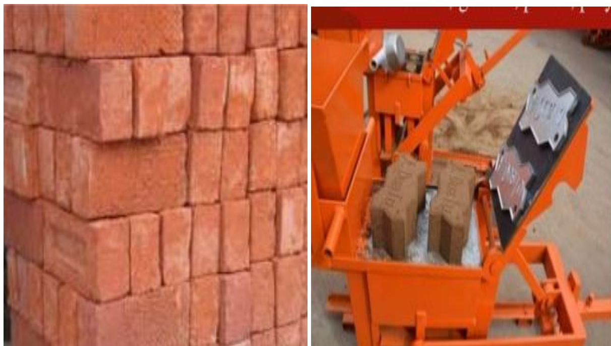
Fig. 4. The red mud clay bricks and biscuits manufactured from red mud
