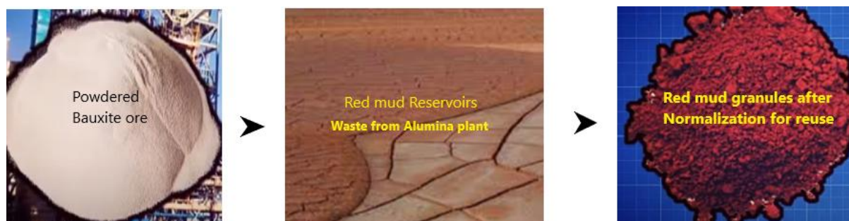
Fig. 1. From powdered bauxite ore to normalized Red Mud for reuse
