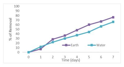
Fig. 7. Bioremediation of Cr (VI) from soil and water contaminated with 297 mg/g soil (pH 6.8), and 400 mg/L Cr (VI) (pH 8.2) (5 g of fungal biomass. 28°C, 100 rpm
