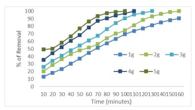
Fig. 4. Effect of initial concentration of the fungal biomass on the bioadsorption of Cr (VI) in aqueous solution.1 g/L of Cr (VI). 100 rpm. pH 1.0
