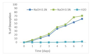
Fig. 6. Desorption of 1.0 g/L of Cr (VI) by different solutions. 28°C.100 rpm. pH 1.0
