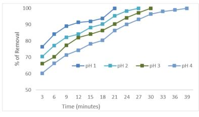
Fig. 2. Effect of pH and incubation time on the bioadsorption of Cr (VI) in aqueous solution by the biomass of *A. bisporus*. 100 mg/L. 1 g of biomass, 28°C 100 rpm
