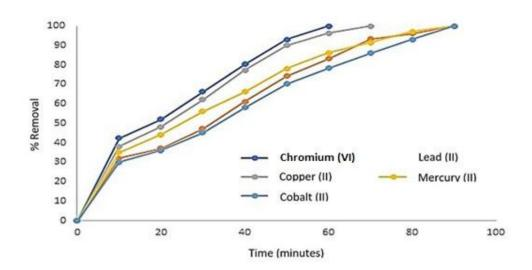
Fig. 5. Effect of the presence of different heavy metals (200 mg/L) on the bioasorption of Cr (VI) in aqueous solution. 200 mg/L of Cr (VI). 28°C.100 rpm. pH 1.0
