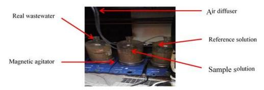
Fig. 1. Biological treatment device using the ZW method
