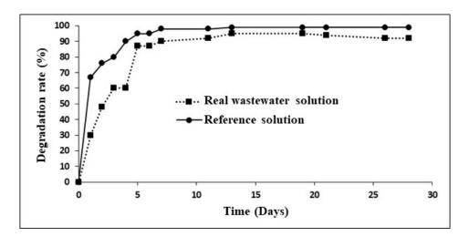
Fig. 2. Rate of degradation of wastewater as a function of time by the ZW; pH = 6.5-8; T = 25 ° C; [activated sludge] = 1.2 g / L; [CH<sub>3</sub>COONa] = 1.2 g / L.
