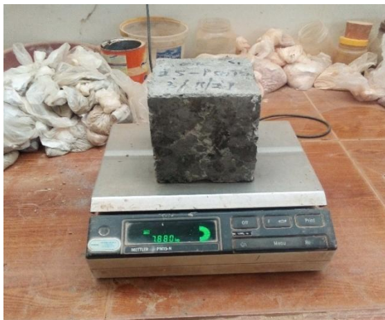
Fig. 3. Measuring the weight of the test specimen
