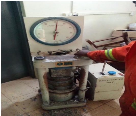
Fig. 2. Compressive strength test
