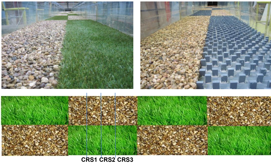
Fig. 2. Two model vegetation simulated with gravel roughness: EXPT1( left upper); EXPT2( right upper) and the plan view showing the three cross sections measured
