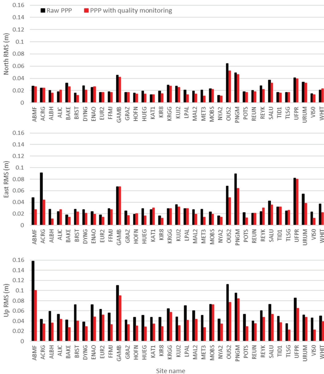
Figure 12. RMS of the difference between kinematic PPP results and the reference coordinates in the north (N), east (E) and up (U) directions for the entire day at 35 stations.
