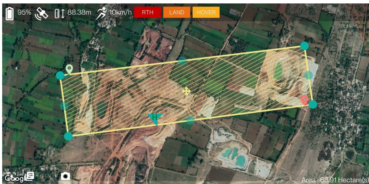
Fig. 3. Drone flying path of the study area mining lease
