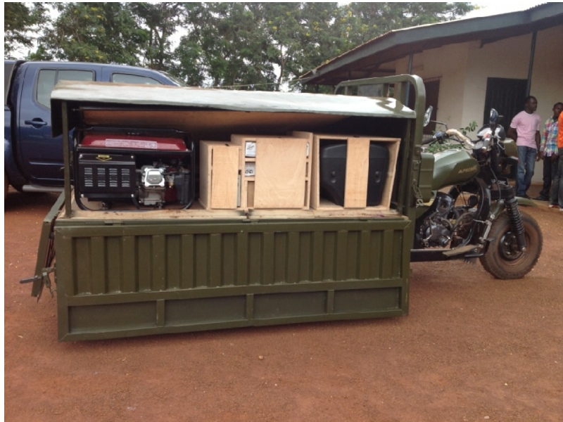
Fig. 2. A motor tricycle modified for ISFM video show
