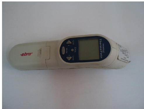
Fig. 8A. Germany non contact temperature measuring device
