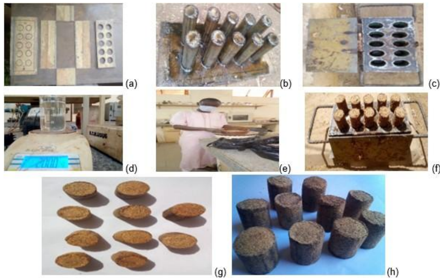
Fig. 1. A cross-section of moulder and briquette making processes: (a) Plate cutting process (b) Base plate (c) Constructed Moulder (d) Water mass measurement (e) Sawdust sieving process (f) Briquette production (g) Sun-drying process (h) Produced briquettes
