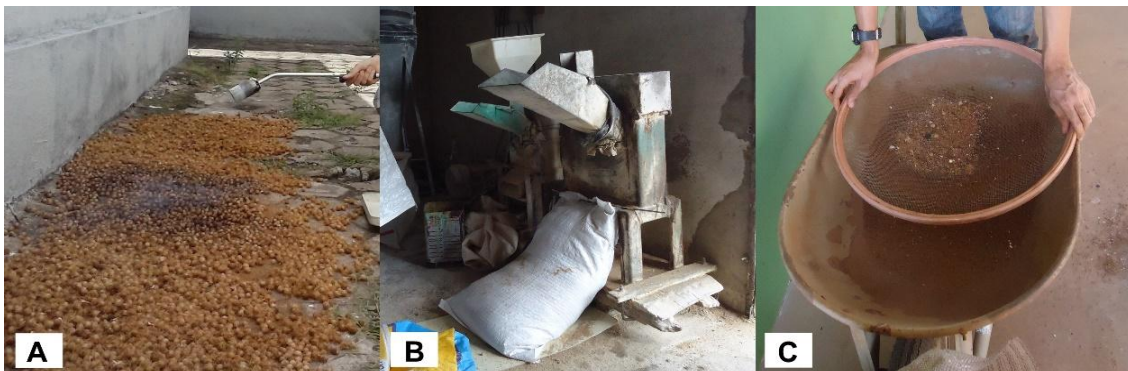
Fig. 2. A - Carbonization of açai berry waste; B - Açai berry waste shredding in a forage; C - Açai berry waste substrate sieving
