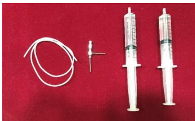
Fig. 1. Co-axial method of electrospinning
