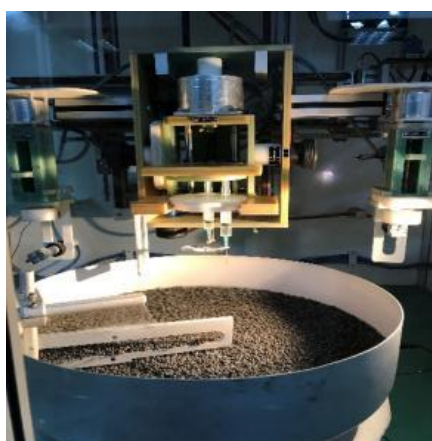
Fig. 2. Vertical electrospinning unit for coating seeds with fibre
