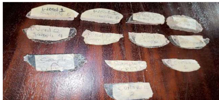
Figure 2. Samples of Some of the composites produced from SD, PE and PET blending.
