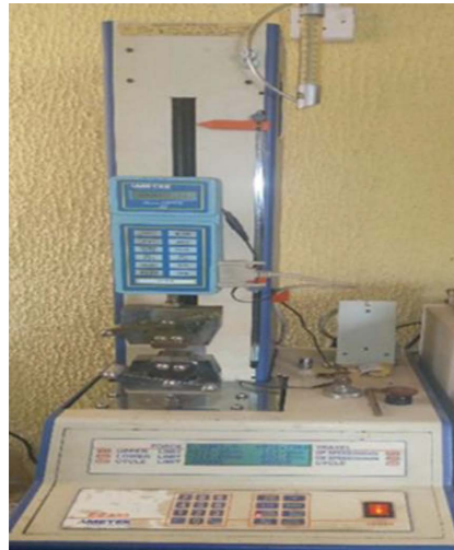
Figure 4. Ametek EZ 250 universal tensile testing machine.
