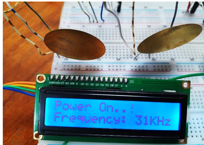
Fig. 10. When the switch is ON, the LCD screen is showing the ultrasonic frequency
