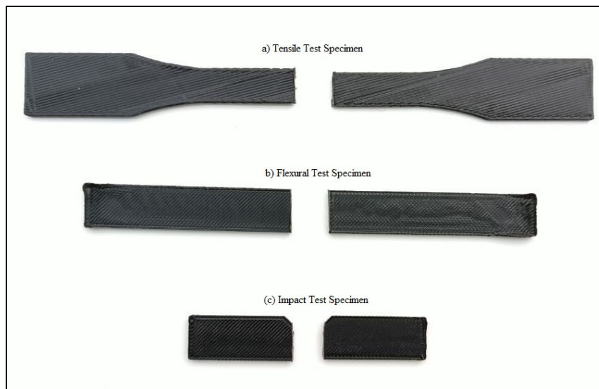
Fig. 2. 3D printed specimens for welding using 3D pen
