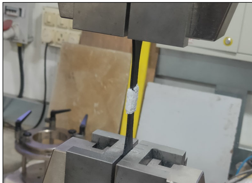
Fig. 5. Tensile testing on the 3D pen welded specimen
