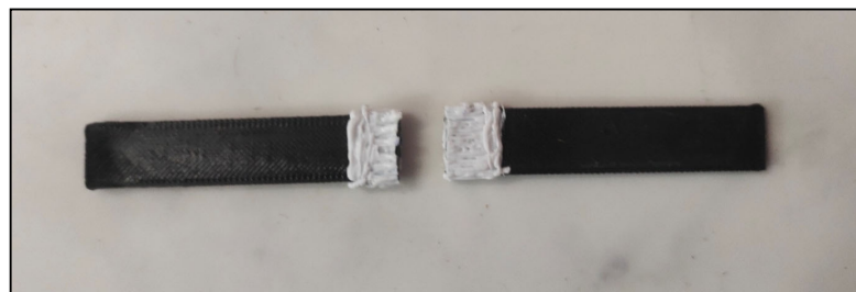
Fig. 7. Failed specimen during flexural test
