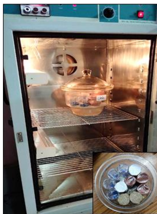
Fig. 2. Experimental Setup for Determination of Water Vapour Permeability of Packaging Materials
