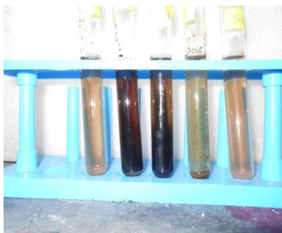
Fig. 1. Indole Test; Test tubes showing dark color (cherry red) indicates indole positive and strain is E. coli and other tubes are negative for indole test
