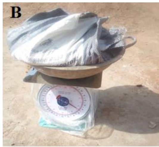
B: Weighing of the stone dust
