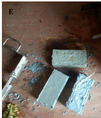
E: Produced stone from nylon plastic wastes
