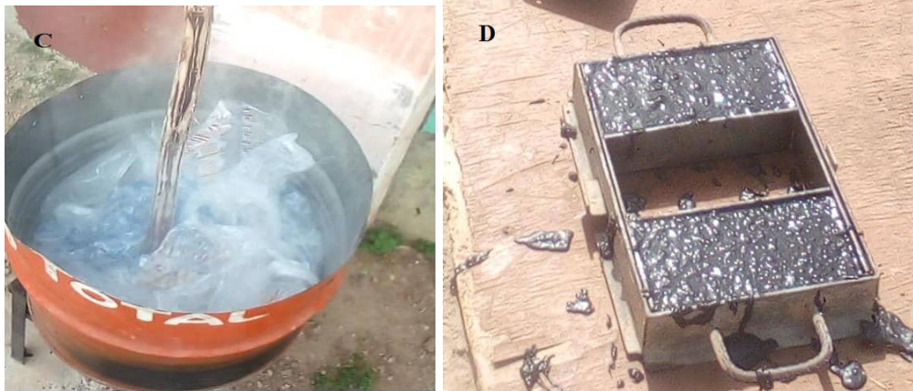
C Melting of nylon on gas burner D Cast melted nylon with stone dust
